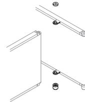
**Four-way joint and adjustable ground foot**
